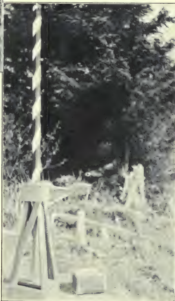
FIG. 8.—THE TYPE OF COMBINATION SIGNAL AND INSTRUMENT STAND USED BY ONE CHIEF OF PARTY WHERE THE LINES WERE SHORT.
